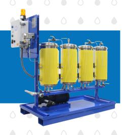
The Model 465-QH is a turnkey filter system designed to handle the high temperatures and heavy particulate loads associated with quench applications. Each COMO Filter holds up to 20 pounds of dirt, so you can extend oil life, improve cooling rates, and achieve uniform hardening with fewer filter changes than the competition.
