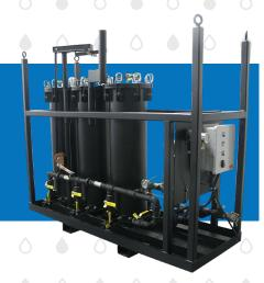
The Model 503 is a turnkey filter system designed for high-flow filtration of large reservoirs up to 7,500 gallons in capacity. The Model 503 utilizes kidney-loop filtration to continuously clean your fluid. With COMO, you can extend fluid and machine life by removing particulate down to 1  $\mu$ m and water contamination to as low as 20 ppm.
