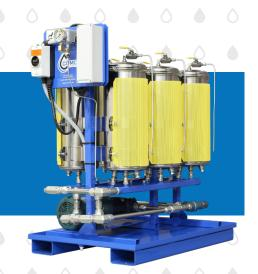
The Model 610-QH is a turnkey filter system designed to handle the high temperatures and heavy particulate loads associated with quench applications. Each COMO Filter holds up to 20 pounds of dirt, so you can extend oil life, improve cooling rates, and achieve uniform hardening with fewer filter changes than the competition.
