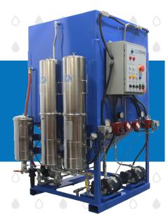
COMO's Oil Recycling Systems reduce filter element consumption by processing batches of contaminated oil through three phases. The heating and settling phases remove most of the water and particulate contamination without loading the filters. Then, the filtration phase polishes the fluid to cleaner-than-new condition.
