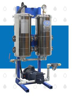
The Model 265 is designed for kidney-loop filtration of a single machine. With dozens of filter options, you can meet your exact cleanliness goals—as low as 1 µm and 20 ppm water. Each COMO Filter holds up to 20 pounds of dirt and 1 gallon of water, so you can extend fluid life and reduce downtime with fewer filter changes than the competition.
