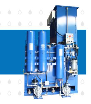
The COMO RTS is a central coolant recycling system that removes tramp oil and particulate contamination simultaneously. By utilizing a split process-tank and two pumps, the COMO RTS keeps dirty coolant additions separate from recycled coolant, thus providing a constant, on-demand supply of clean coolant.
