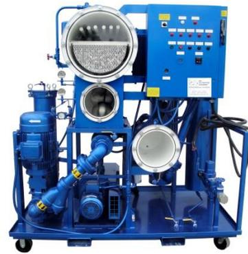
**Results:** The starting varnish content in the oil was MPC 35.2 on December 16, 2015, and an earlier oil analysis had revealed a water content of 292 PPM and an ISO Cleanliness Level of 21/20/17. After 30-days of run time, the varnish content dropped to MPC 11.3, the water content was measured at 0 PPM, and the ISO Cleanliness Level was 19/17/15.
