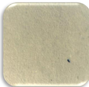
Patch Test Results Brand New Oil In Tote (After Filtration) ISO 16/14/11
