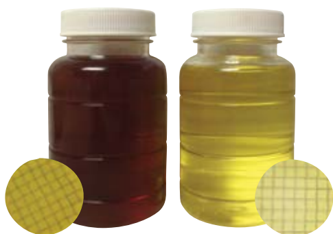
Before Filtration ISO 21/20/17 MPC* Value = 35.2
