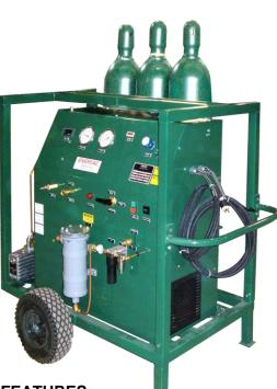
We developed the GRU-7 for our customers who found they needed more storage and recovery capacity than smaller handcart mounted units, but without the bulk and high price of a large skid or trailer-mounted unit.
