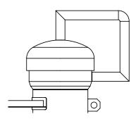
The quick open threaded hinged closure uses a cap fastened to a hub and is welded to the strainer body. The female cap is threaded onto the male hub using O-rings to seal. The O-ring prevents corrosion of the closure threads and provides a long, trouble free service. The threaded cover can be used for both nominal and high pressure applications. Available in both vertical and horizontal configurations.
