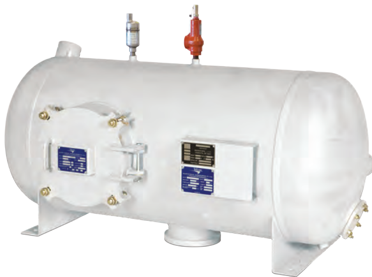
Model No. HVS2228M A fully-qualified 510 USGPM Filter/Separator. Side Opening unit is only 22 inches in diameter and 65 inches long.
