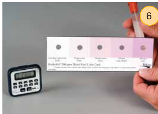
If color is the same or darker than FAIL, more than 200 ppm of free water is present.
