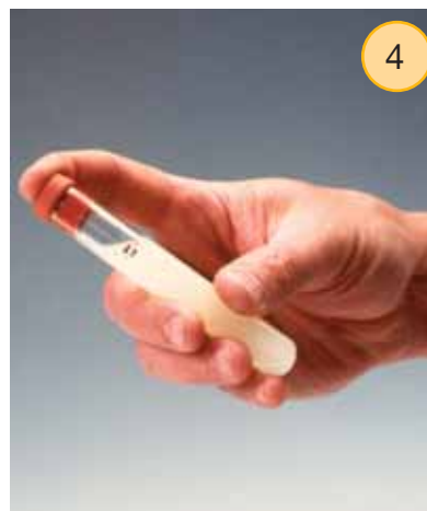
After tube fills, shake for 15 seconds. Set upright to allow powder to settle.
